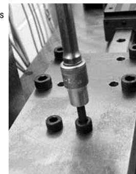
7. Vent compressed air, the system will align itself, tighten screws to the required torque setting (table 1), process should be conducted gradually.
